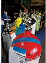
Any cylinder that fails a visual inspection, hydrostatic requalification or eddy-current test should be neither
